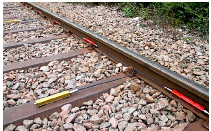
Efficient installation with the latest generation of sensors! Amberg TrackControl Pro with flexible plug connections and innovative magnet fastening.
