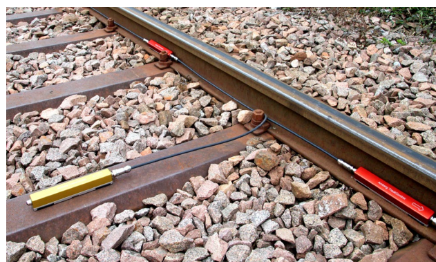
Efficient installation with the latest generation of sensors! Amberg TrackControl with flexible plug connections and innovative magnet fastening.
