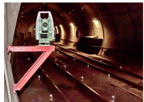
Track monitoring with total station
